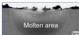
Fig.3 Molten pool observation by X-ray (Spring-8)
